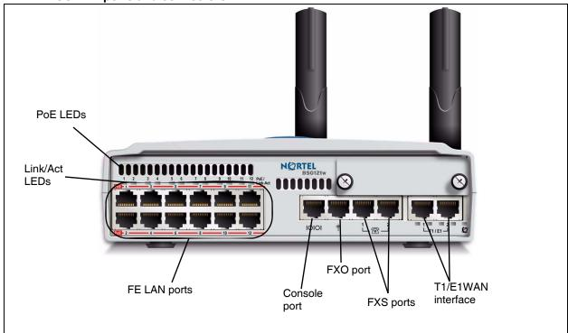
The BSG12ew has eleven FE LAN ports. For this unit, the twelfth port is used as the FE WAN interface. For BSG12ew ports and connectors, see "BSG12ew ports and connectors" on page 16.
